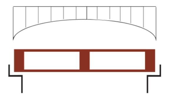
Load bridging is the redistribution of load weight away from the center of the pallet
