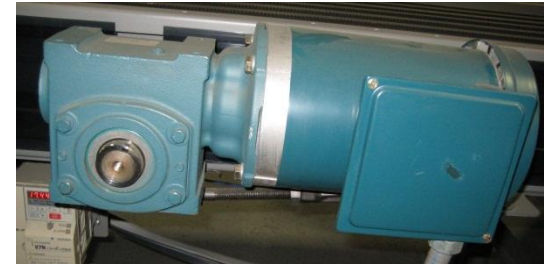
Direct drive eliminates chain and belts
