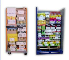
The order pallet is built inside a three-sided frame for added stability.
