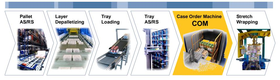
Fully automated storage and picking process using standard automation technology throughout the design
