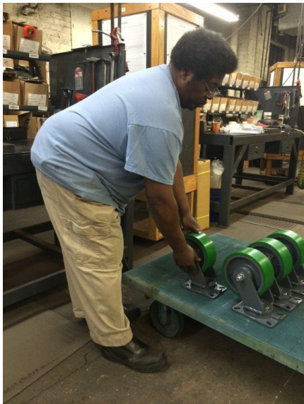
Platform too low
